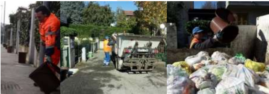
Figure 11: A non-compacting vehicle with single driver, for the manual collection of food waste in buckets
